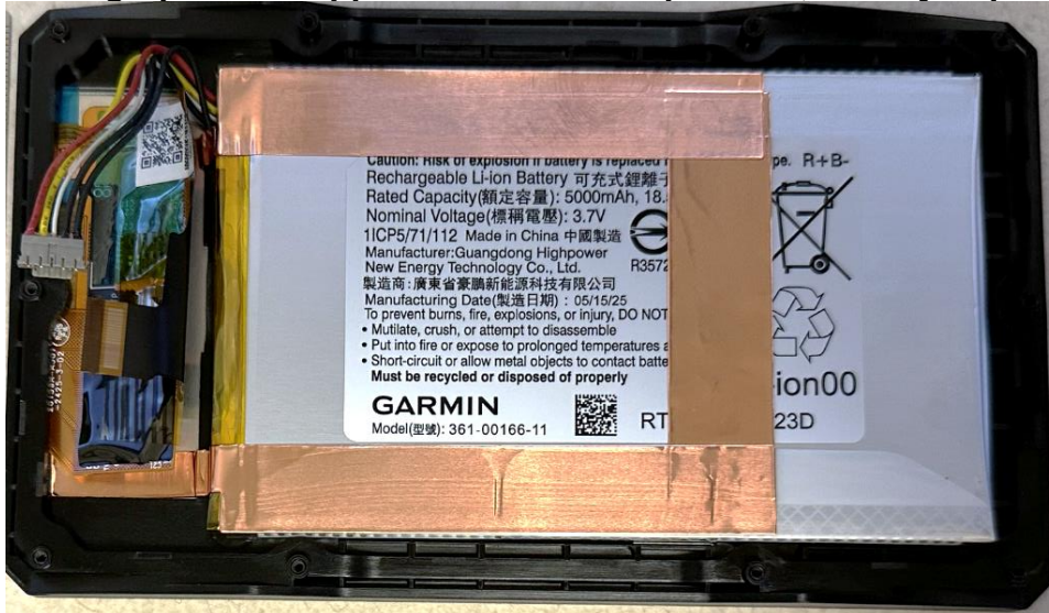
Photograph 07-6: Upper enclosure components, battery in place
